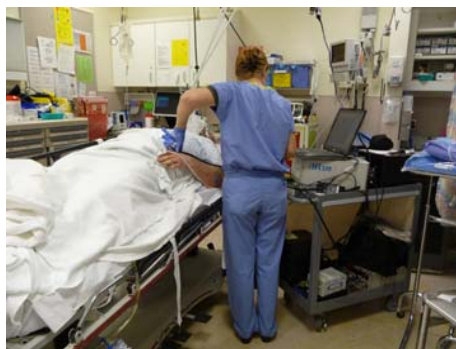
Fig. 3. Prototype shock monitor in the Emergency Department at Harborview Medical Center measuring muscle oxygenation in a trauma patient
